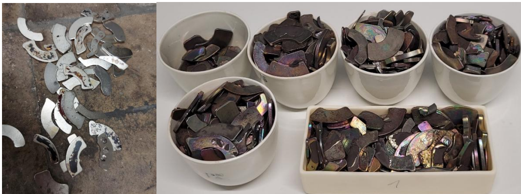
Figure 3 Magnets demagnetization by thermal treatment.
