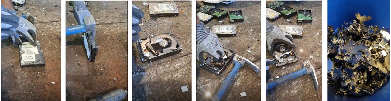
Figure 2 The collected FeNdB-magnets from HDDs were disassembled manually.
